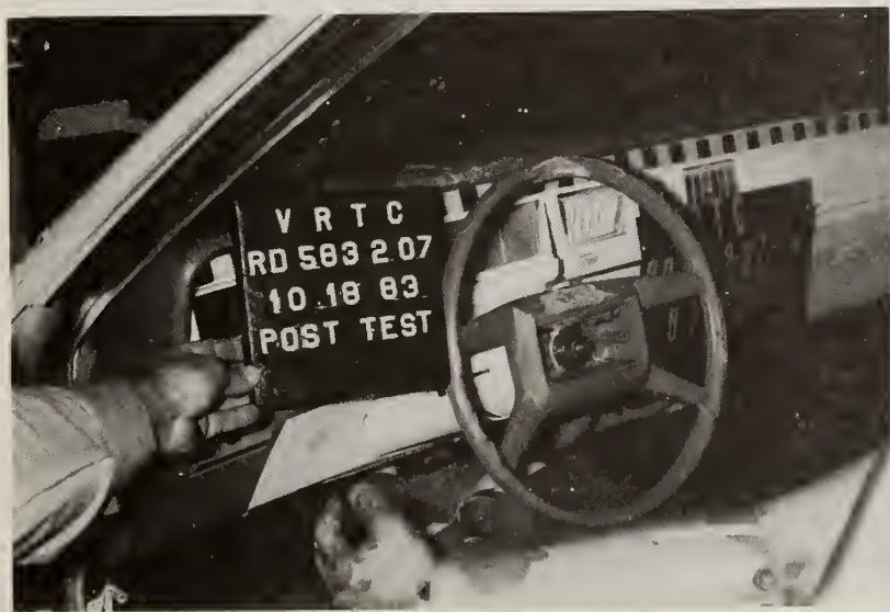
Steering Wheel Deformation, Left View Test 7
